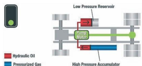
Figure 2: Releasing energy during acceleration.
