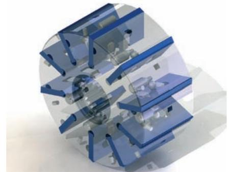
Figure 5: Transparent rotor showing vane restraint.
